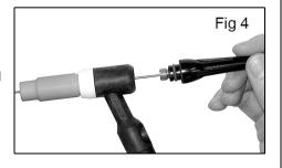
move, adjust it so that it protrudes from the nozzle by 4 - 5mm, and then tighten the end cap against the rubber O-ring. The electrode will now be secured in position. Your torch assembly is now ready for use.
